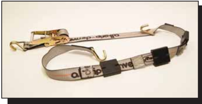
PART NO. 804SHDH1 7.2 lbs. This strap goes over the wheel and comes with wire hooks, two fixed and one floating. Three rubber cleats engage and are retained within the tread of the tire. Tightening the supplied ratchet secures the wheel to the deck. W.L.L. is 3,335 lbs.
