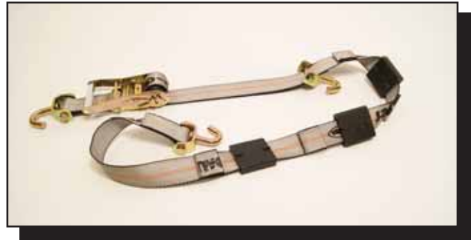
PART NO. 804SHDH2 7.4 lbs. This strap goes over the wheel and comes with swivel type finger hooks, two fixed and one floating. Three rubber cleats engage and are retained within the tread of the tire. Tightening the supplied ratchet secures the wheel to the deck. W.L.L. is 3,335 lbs.
