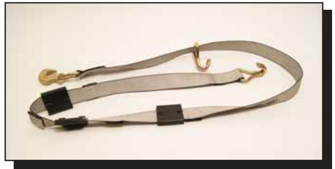
PART NO. 4821HDH4 6.2 lbs. This strap goes over the wheel and comes with 2 wire hooks, one fixed and one floating. Three rubber cleats engage and are retained within the tread of the tire. The other end has a fixed grab hook for attachment to your existing chain and chain winch. W.L.L. is 3,335 lbs.
