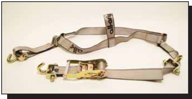
PART NO. 804SHDH3 7.1 lbs. This strap baskets the wheel and comes with swivel type finger hooks, two fixed and one floating. Tightening the supplied ratchet pulls the basket down tight, securing the wheel to the deck. W.L.L. is 3,335 lbs.
