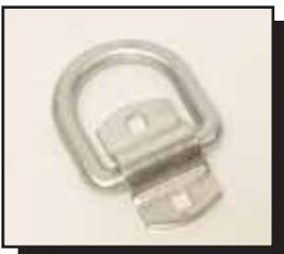
These tiedown rings are for carrier mounting. They make great anchor points when secured correctly. They use (2) 3/8"x3" grade 8 carriage bolts. (Not Supplied)
